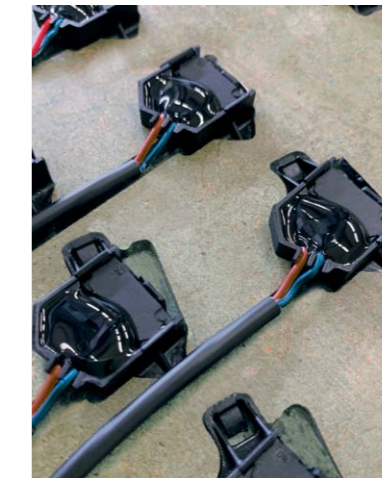
Dispensing on micro switches.
