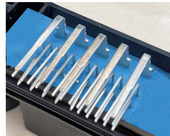
Potting on connectors.
